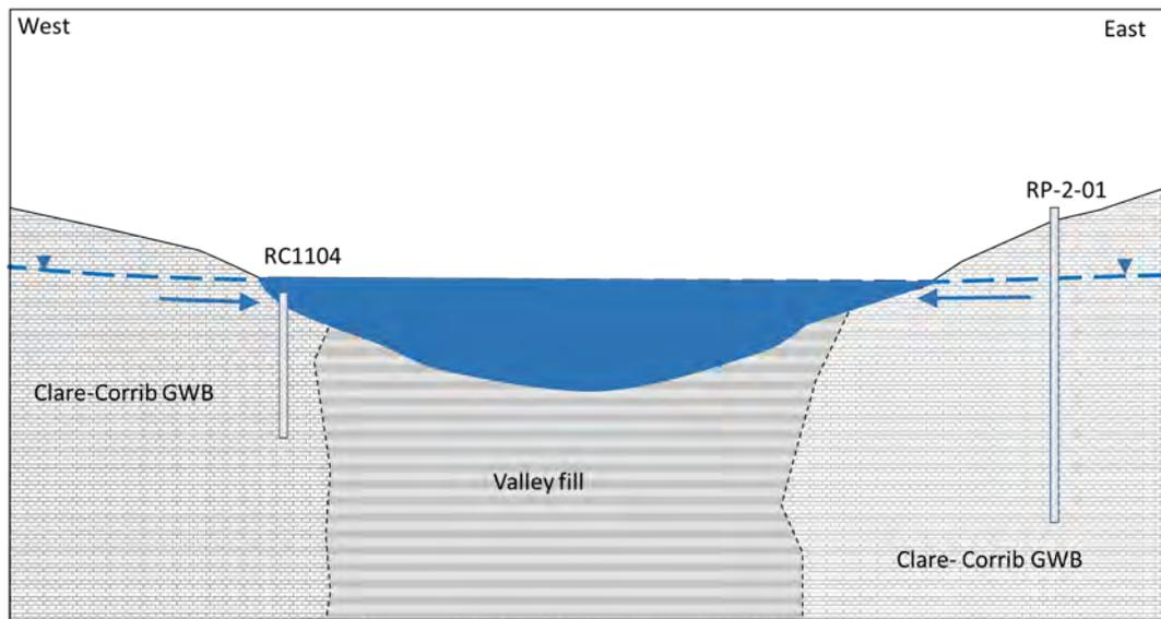
**Plate 7: Schematic east west cross-section through Ballindooley Lough showing the interaction of groundwater with the lake during low groundwater levels**
