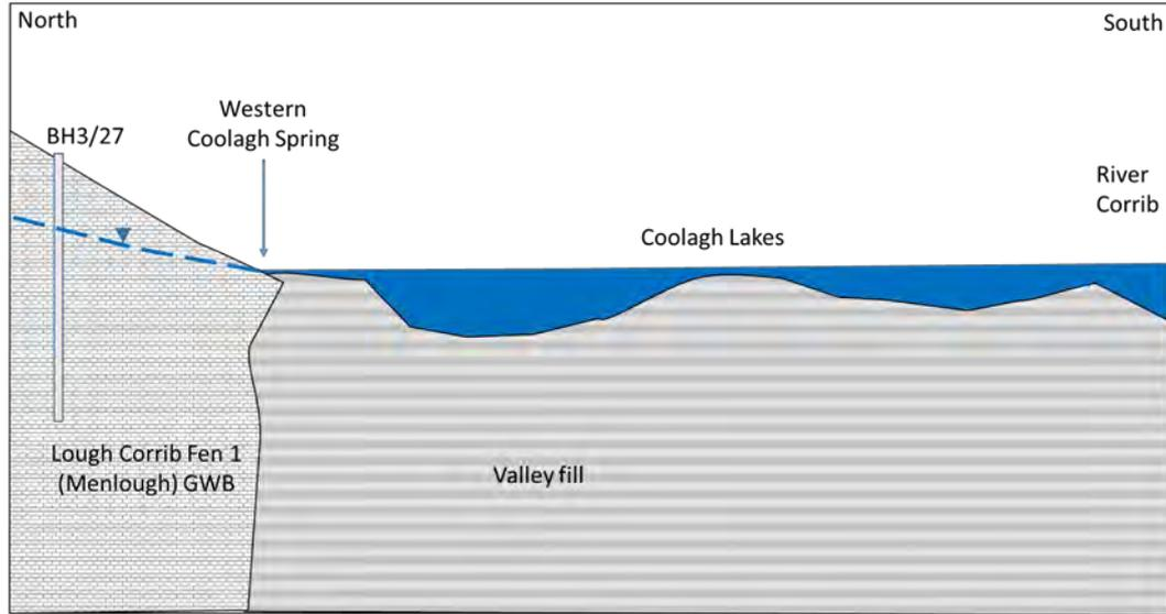
**Plate 4: Schematic north south cross-section through Coolagh Lakes (groundwater low)**
